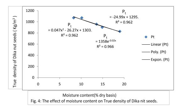
The true density varied from 1071.75 to 901.80 kg/m<sup>3</sup> when the moisture level increased from 8.25 to 18.98% (dry basis) Figure. 4 The true density and the moisture content of seed can be correlated as follows
