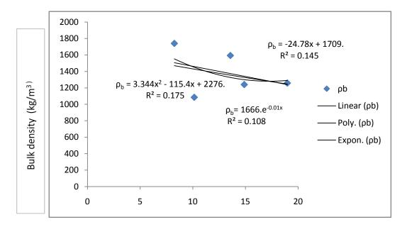
Moisture content (% dry basis) Fig. 3: Effect of moisture content on bulk density of Dika nut seeds.
