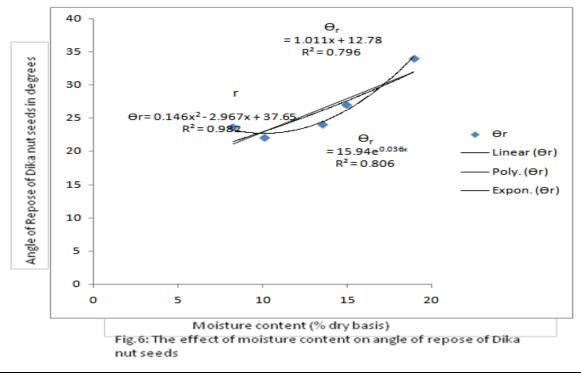
$\begin{array}{l} \mbox{The angle of repose of the Dika nut seeds and the moisture content of seed can be correlated as follows:} \\ \Theta_r = 0.146 x^2 - 2.967 x + 37.65 \\ \mbox{R}^2 = 0.982 \\ \mbox{(19)} \end{array}$
