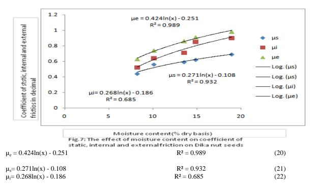
The increase in static friction with increase in moisture content (Altuntas and Dermirtola, (2007) may be due to increase adhesion between the seeds and the surface at higher moisture levels.
