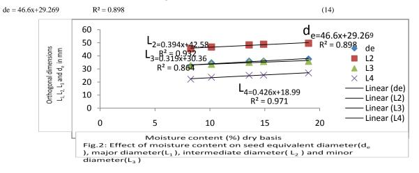
The increases in L1, L2, L3 and Le with increase in moisture from 8.25% dry basis to 10.14% dry basis were 34.62, 46.72, 33.60 and 23.56% respectively. These values also increased as the moisture contents were increased through 18.98% dry basis. Karimi *et al.*,(2009) and Sadeghi
